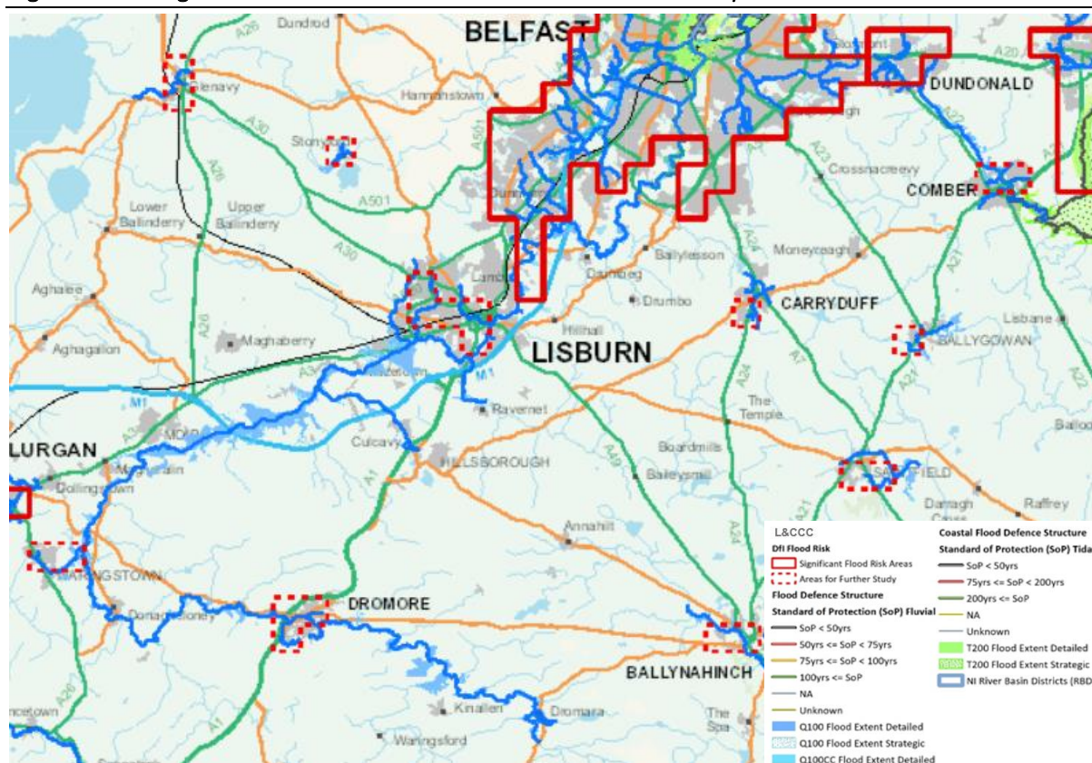
Figure 5.11.5: Significant Flood Risk Areas and Areas for Further Study with River & Coastal Flood Plain
